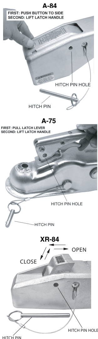
FIGURE 5 OPENING COUPLERS
